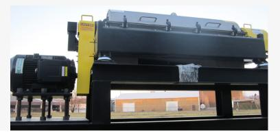
A long-term Kroeschell client has an ongoing need for new machinery to be installed and old machines to be relocated within a 1-million-sf. facility. The machines account for nearly 95% of the total production facility onsite. Work for this project has included laying and painting foundations, safely delivering and placing machines, installing wiring, air, and water connections, and ensuring proper operation while safely and efficiently relocating or removing old machinery.
